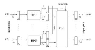
Figure 3. Block diagram showing the micro-architecture of a synchronous TDM router. The design is a 3-stage pipeline: (i) link traversal, (ii) header parsing unit (HPU) and (iii) traversal of the crossbar switch (Xbar)
