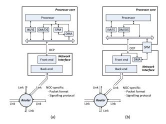
Figure 2. (a) Block-diagram showing the conventional architecture of processor node. The figure expands the view of Fig. 1. (b) Block-diagram using the new area-efficient NI-design presented in [24].
