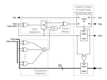
Figure 7. Circuit implementation of the LEDR to 2-phase bundled-data converter – the first pipeline stage of the router.
