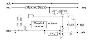
Figure 4. Diagram of the HPU implementation in the asynchronous designs.
