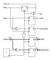
Figure 9. Circuit diagram of Bundled-data to LEDR converter [27].
