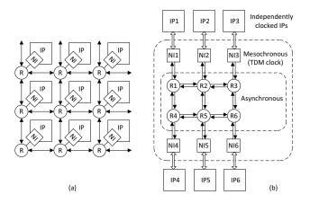
Figure 1. (a) Structural organization of a generic NOC-based multi-core platform. (b) Timing organization of a platform using the asynchronous timedivision-multiplexed NOC explored in this paper.
